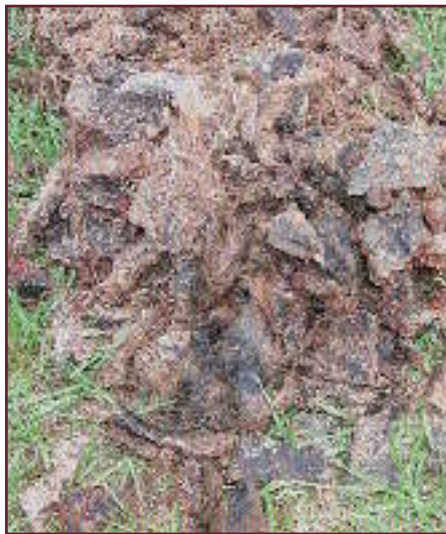
Top: Tire chips before installation. Bottom: Tire chips excavated from system eight years later shows growth of biofilm and lack of tire chip decomposition. Photos courtesy of Barbara Grimes.
